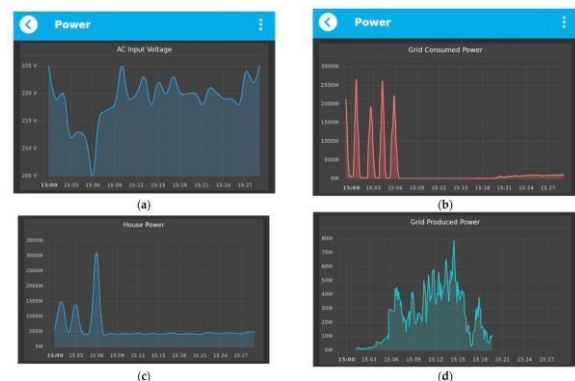
Figure 3: An example of monitoring the power with qToggle: AC Input Voltage (a); House Power (b); Grid Consumed Power (c); Grid Produced Power (d).[1]
