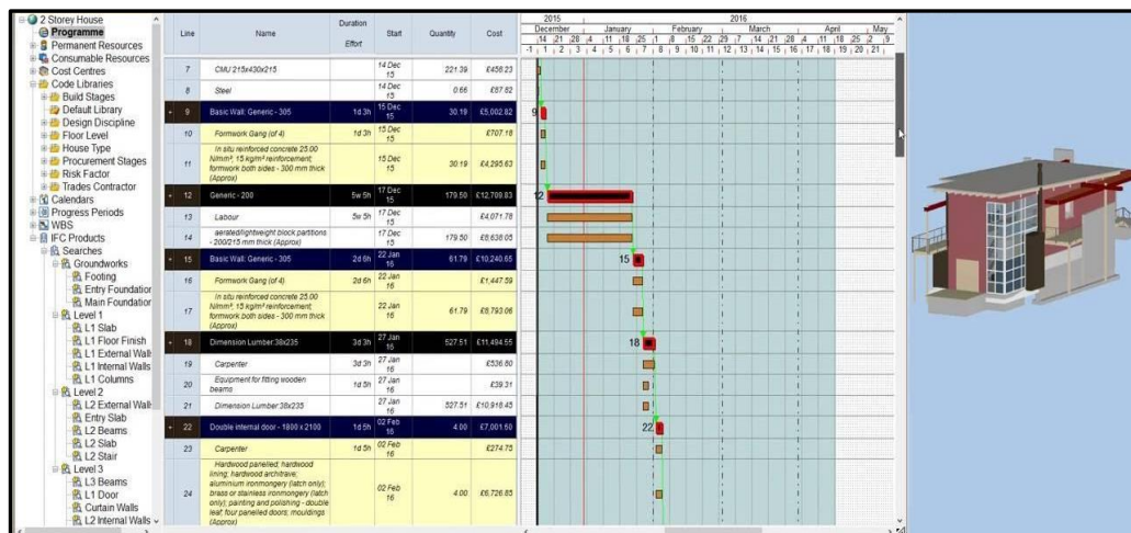
Figure 11. 5D BIM-EVM Illustration (Synchro Construction, 2017).
