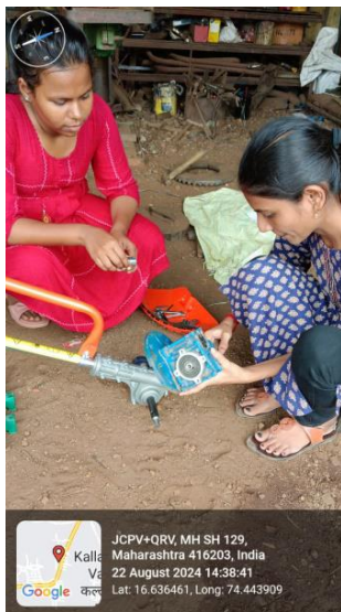
Fig no. 10- Fixing of Gear box
