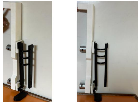
Fig.10 Isometric view (Left) and Front view (Right) of the fabricated prototype
