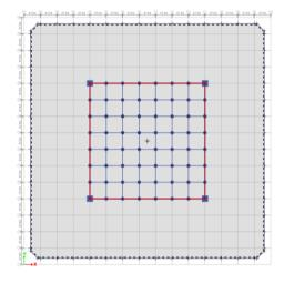
Figure:2 Top View for the 5% tapering Combined with chamfered edge modification
