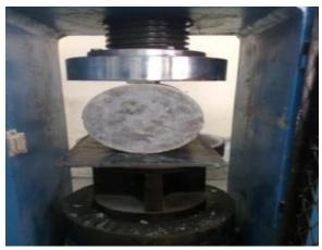
RESULT:-We obtained that when we replace cement with Rice husk ash, we get maximum tensile strength at 15%. To further increase the tensile strength of concrete, we added steel fiber to it because concrete is strong in compression but weak in tension, so we replace cement with 15% Rice husk ash and added some percentage of steel fiber (0.5%, 1.0%, 1,5% and 2.0%) to it. Hence, we get more Tensile strength than Rice husk ash mix concrete.
