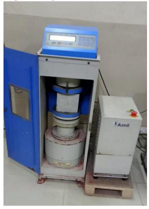
TENSILE STRENGTH:- Split Tensile strength is the important property of concrete .we know that concrete is strong in compression but weak in tension. That's why we have used steel fibers to increase the tensile strength of our concrete. In the present study 7 & 28 days split tensile strength of cylinder specimens of (150mm dia & 300mm length) have checked.
