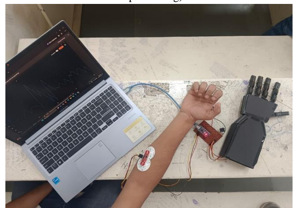
Figure 4. Final Prototype (including EMG sensor, 3D printed arm, microcontroller, circuit working, output waveforms, etc.)
