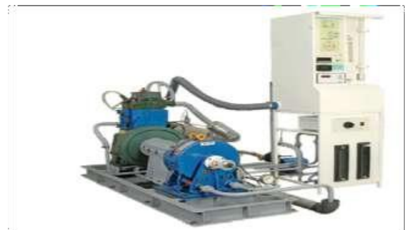
Fig-4: Computerized Single cylinder 4 stroke Diesel engine(VCR engine)
