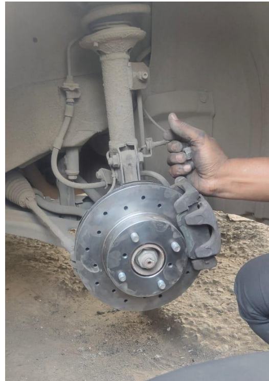
Figure 12: Ventiladed Disk Rotor with 7 mm cross Drill mounted on Wagon R
