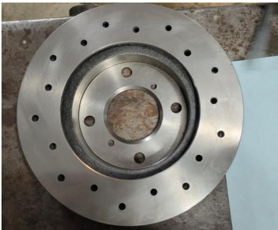
Figure 11: Ventiladed Disk Rotor with 7 mm cross Drill
