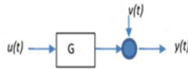
Fig.1 A linear Time Invariant System with disturbance
