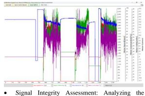
Signal integrity Assessment: Analyzing the drone's frequency data allows investigators to evaluate the stability of communication during the flight, helping to identify potential communication failures or signal disruptions that could have affected the flight.
