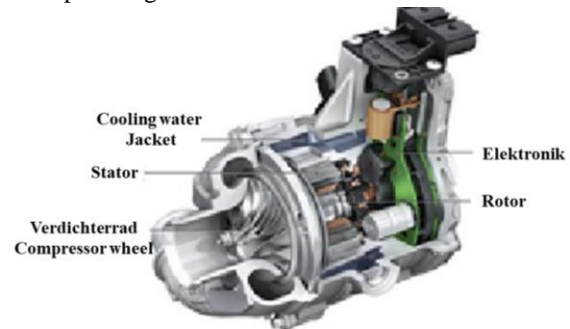
Figure 3.2 Section views of Electrical Superchargers
