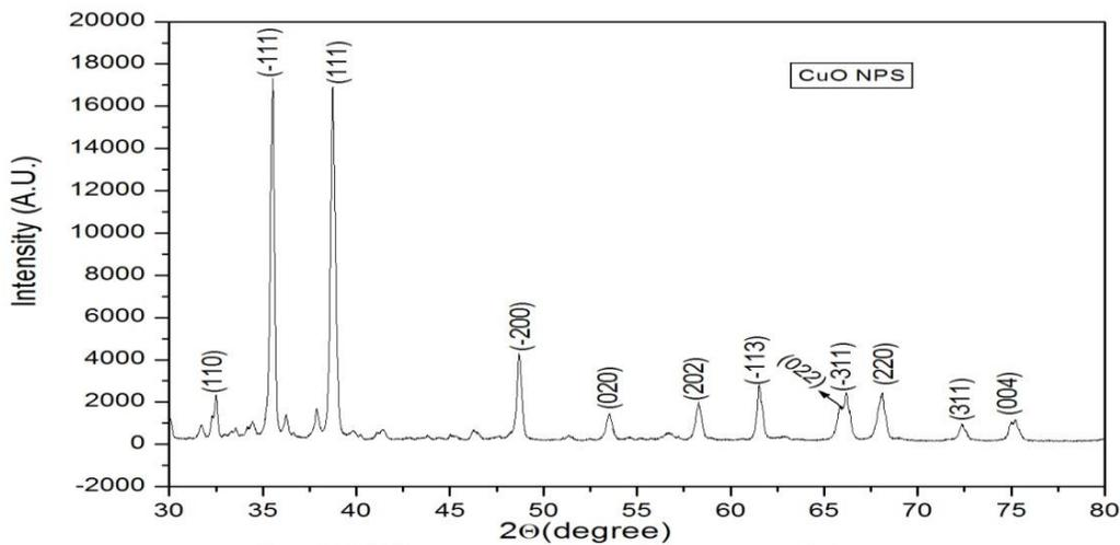
Fig.2 XRD pattern for CuO nanoparticles
