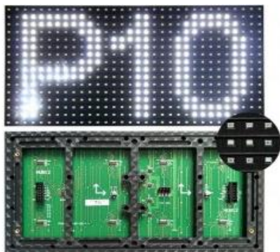
Figure 2. Frontal and back view of Four 64x32- P10- RGB-LED panels
