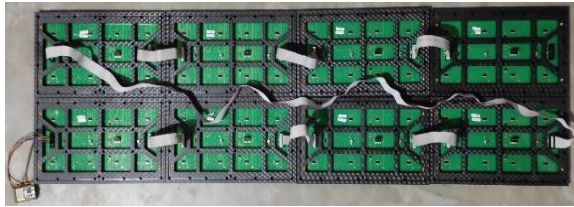
Figure 5. Connection between HUB75 interface and P10 panels
