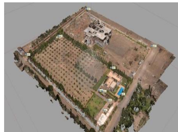
Figure 6. Orthophoto with a ground sample distance of 3cm
