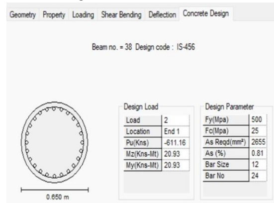
Fig 4.5.5.1: Design of column
