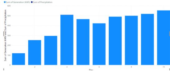
Graph depicting the relationship between precipitation and solar generation. Despite the short-term reduction in generation during rain, subsequent periods show increased performance due to the cleaning effect of precipitation.
