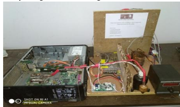
Fig.01.VCR System for CPU Cooling
