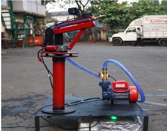
Fig.1.1 360-degree rotating fire protection system
