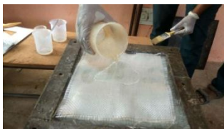
Fig-1 Specimen fabrication by hand lay-up
