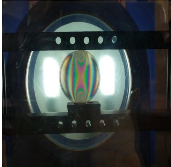
Figure 4.7 Fringe pattern of Calibration disc in white light source
