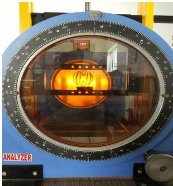
Figure 6 Fringe pattern of Calibration disc in monochromatic light source
