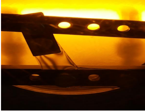
Figure 8. Bell crank lever at 120° in Circular polariscope
