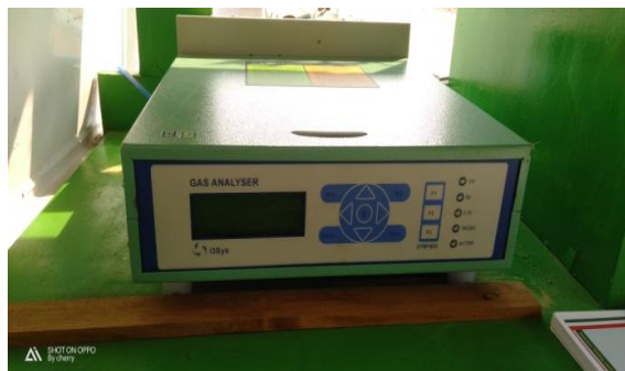
Fig.4.2. Exhaust Gas Analyzer
