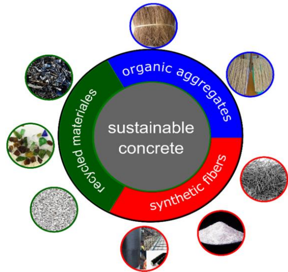
Fig. 1: Various materials can be used for the production of sustainable concrete [16]
