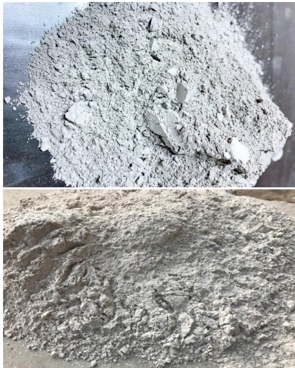
Figure 1: Raw cement sample and fly ash sample Aggregates are categorized as either 'coarse' or 'fine'. Coarse aggregates consist of particles larger than 4.75mm, typically falling within the range of 9.5mm to 37.5mm in diameter. Fine aggregates, on the other hand, generally comprise sand or crushed stone with a diameter less than 9.55mm. Locally available fine and coarse aggregates used in the production of self-
