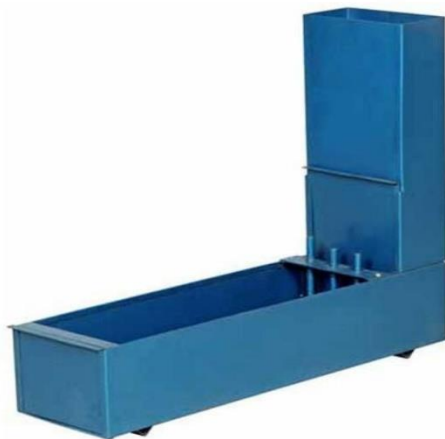
Figure 3: L-box test on fresh SCC
