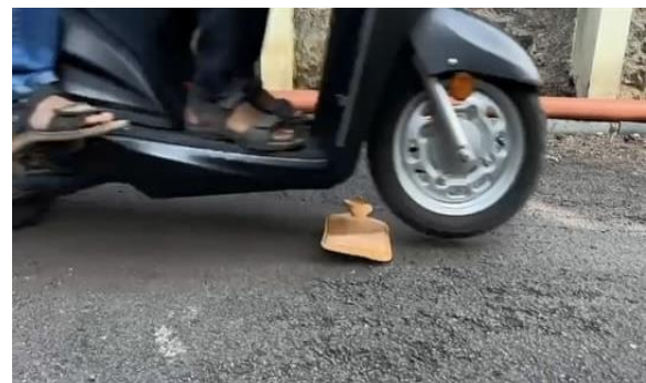
Fig 6: Resistance Test Using Heating Bag Under Bike Load
