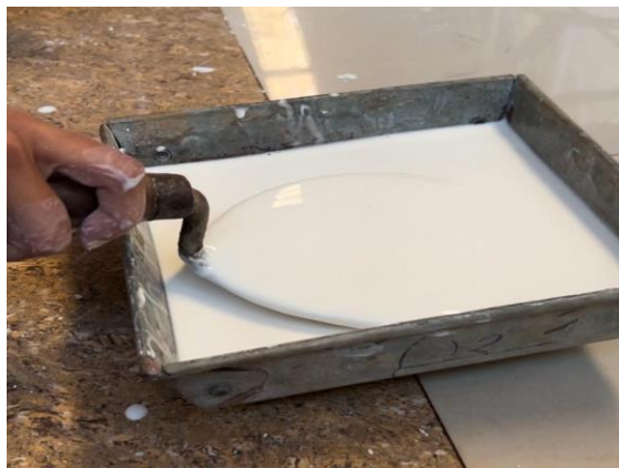
Fig 3: Shear-Thickening Effect Demonstration
