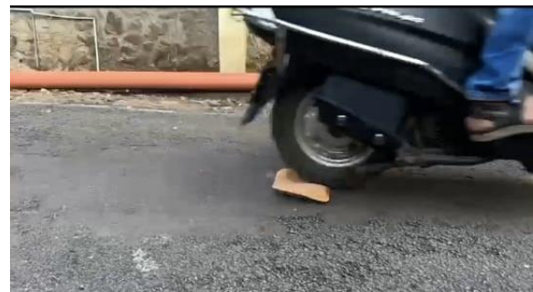
Fig 5: Resistance Test Using Heating Bag Under Bike Load
