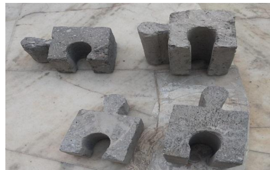
Fig 1 New Developed Mortar-Less Interlocking Wall Block
