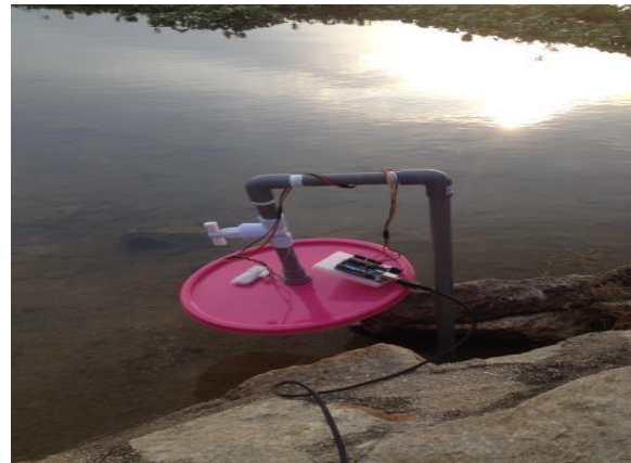
Figure 4.12 Ultrasonic sensor outdoor test
