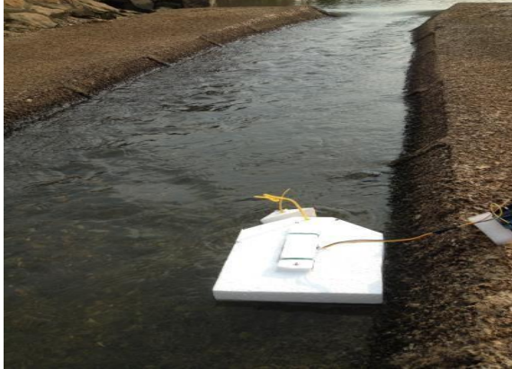
Figure 4.10 Water flow sensor outdoor test
