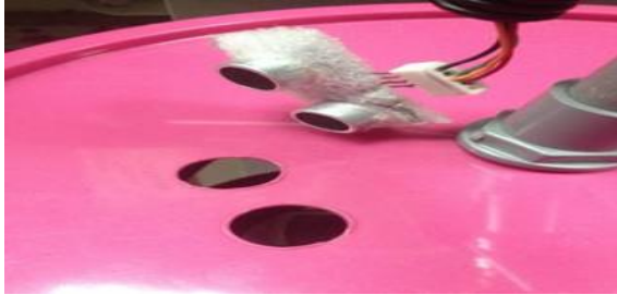
Figure 4.15 Ultrasonic sensor (wired) Subsystem Integration (Wireless)
