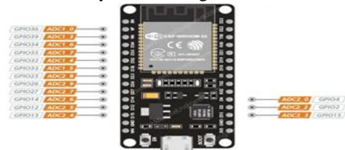
Figure. 2. Analog pin diagram of ESP32 controller
