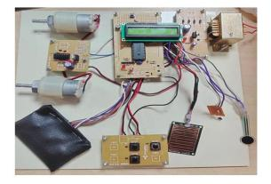
By combining sweat detection, air circulation, temperature and pressure monitoring, and real-time data processing, the system ensures optimal patient comfort and skin health.
