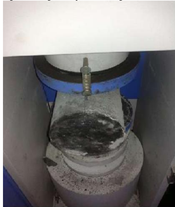
Fig 4.7 Testing split tensile strength.
