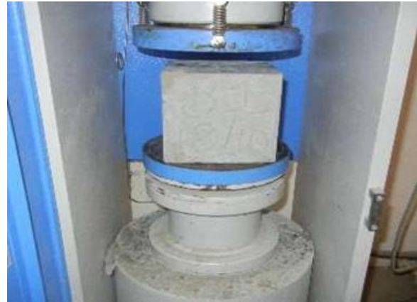
Fig 4.6 Testing of compressive strength.
