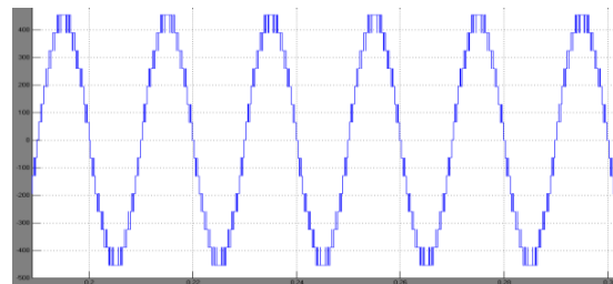
Fig.9 Output wave for 18 switch MLI inverter output voltage with 15 level of waveform
