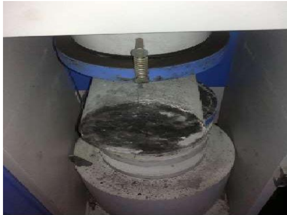
Fig 4.8 Testing of split tensile strength
