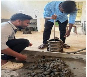
component materials. seasoning, for illustration, bond and M- sand are blended, to which the fine total and coarse aggregate are included and fully blended. Water and Glass fibers are measured precisely. At that point it is added to the dry mix and it's fully blended until a mix of even shading and thickness is fulfilled which is also prepared for throwing. Before throwing of samples, workability is measured as per the code IS 1199- 1959 by droop and compaction variable tests.
