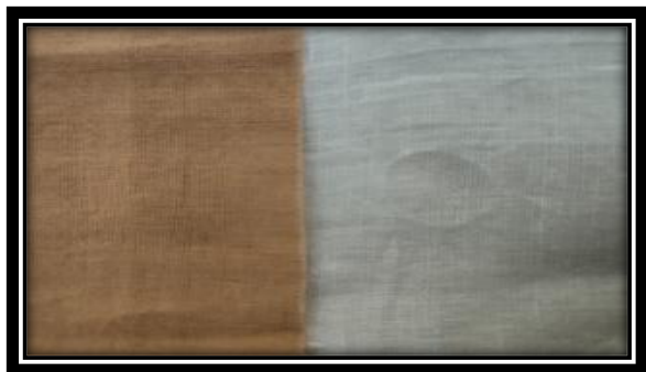
Fig.3 By Crocking [wet] sample there was no colour Bleed onto the Undyed Fabric
