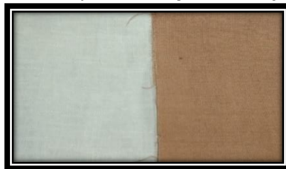
Fig.1 By Ironing there was no Colour Bleed onto the Undyed Fabric
