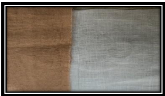
Fig.4 By Crocking [Dry] sample there was no colour Bleed onto the Undyed Fabric
