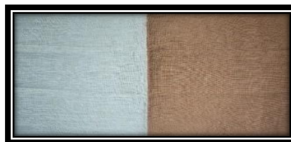
Fig.2 By Washing there was no colour Bleed onto the Undyed Fabric
