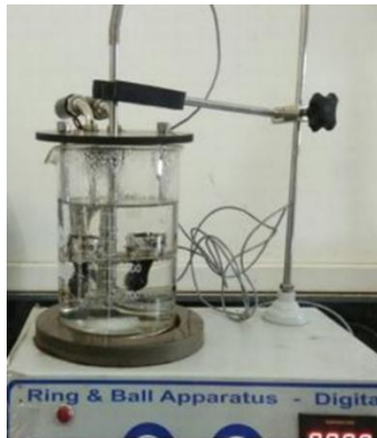
Figure 24: Softening point Setup
