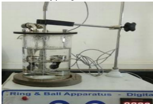
Figure 24: Softening point Setup
