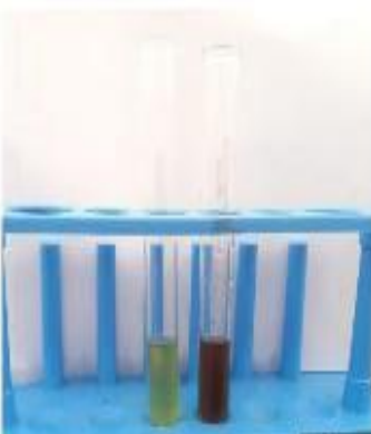
5. Phenols test - positive
