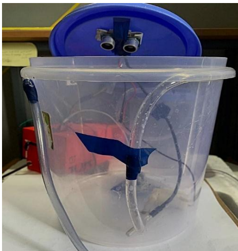
Fig 7: Ultrasonic sensor attached to the miniature main tank
