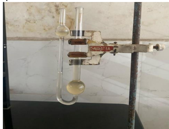
Figure.No.17Rheological evaluation with oswalds viscometer
