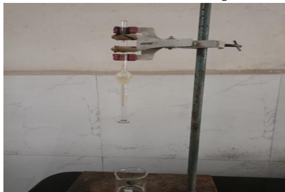
Figure.No.18 Surface tension determination of shampoo with Stalagmometer
