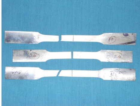
Fig.10 Tensile specimens of welded joints
