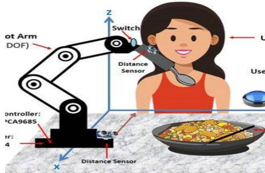
Fig 5: Intelligent Food-Feeding Arm for Individuals with Disabilities Using ESP32 and Servo Motors
