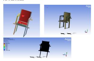
Nodes-1239531: The number of nodes in the mesh refers to the finite element method points where displacements, stresses, and other results are computed. The higher the number, the finer the mesh will be, which is usually the case for accurate results.
