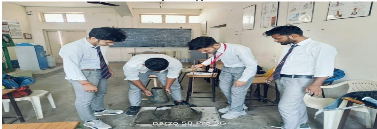
Slump height begins checked after removal of mould
