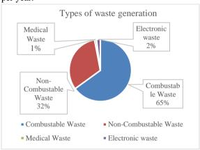
The waste generation per year is 12,140 metric ton.By process this waste it only generates 0.438MW
