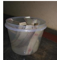
Fig6 (d): The Specimens of 0^\circ/90^\circ Orientation are immersion in the water
