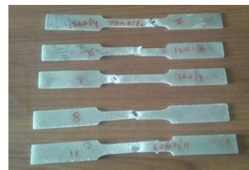
Fig 7: The Specimens after Tensile test
