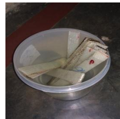
Fig6(c): The Specimens of 60^\circ Orientation are immersion in the water
