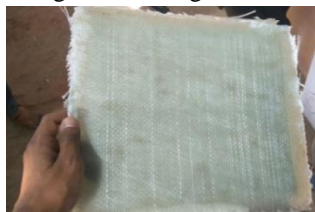
Fig 3: Final Composite laminate
