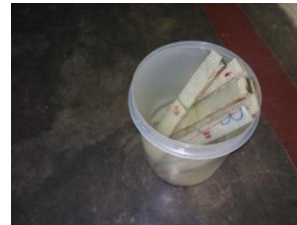
Fig 6(b): The Specimens of 45^\circ Orientation are immersion in the water
