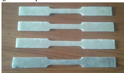
Fig 5: The Specimens before Tensile test
