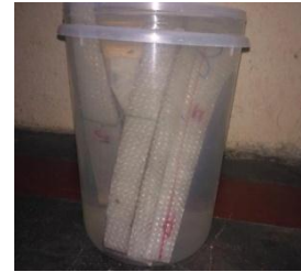
Fig6(a): The Specimens of 30^\circ Orientation are immersion in the water
