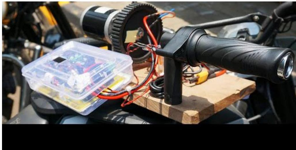
It compares the actual speed with the desired speed (from throttle) and adjusts PWM duty cycle accordingly to maintain a stable output (feedback control).
