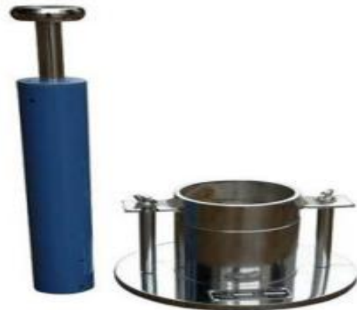
Fig 3.1. Modified Proctor test apparatus
