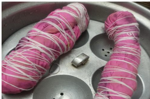
Fig:11 Bundling the flowers using thread And steaming it in the pre-heated in Vessel
