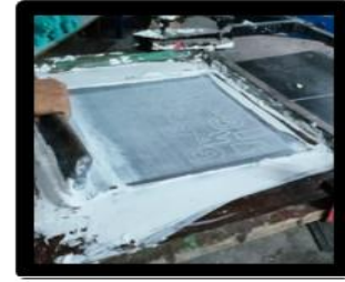
Figure 07 (Spread the pigment through the screen using the squeegee)
