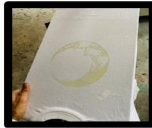
Figure 08 (The pigment is transferred through the screen in fabric)
