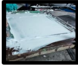
Figure 06 (Apply the pigment in the screen)
