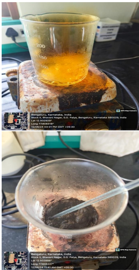
Fig 17: Acid digestion of filtered water sample and biochar to determine cadmium concentration
